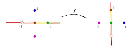
Next, we may try to find the image of the y-axis. So, one may calculate  $f(\mathbf{i}y) = u + \mathbf{i}v$ . Then, it can be checked that  $u^2 + v^2 = 1$ . That is, the image of the y-axis lies in the unit circle. More details can be observed by showing (as an exercise) that
